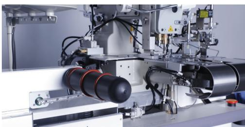
**Equipped with deviation correction, edge folding, and stitching alignment mechanisms. Simplified operation only requiring operators fitting the bottom side to the**
